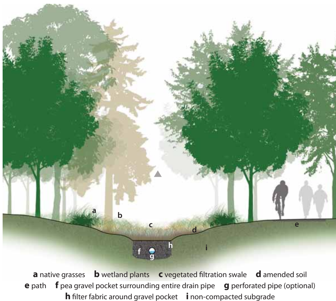
Figure 39: Schematic Section of a Bioswale
